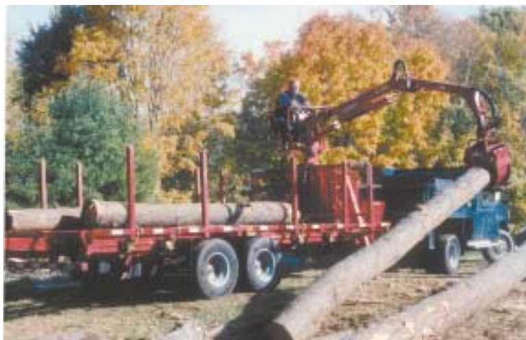
Richard Brown has added a hydraulically operated winch to his Wheeler trailer and Métavic loader combo.
